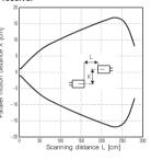
•2mm wide vertical slit mounted at both emitter and receiver
