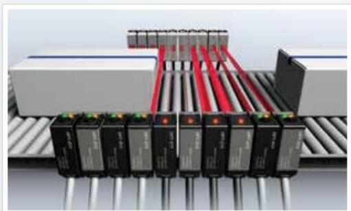
Use when switches need to be closely packed to judge workpiece size, etc. The combined use of standard and different-frequency switches and the mutual interference protection filter enables serial installation of multiple switches.
