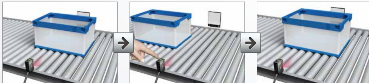
Light passes through semi-transparent target objects, affecting detection consistency.
