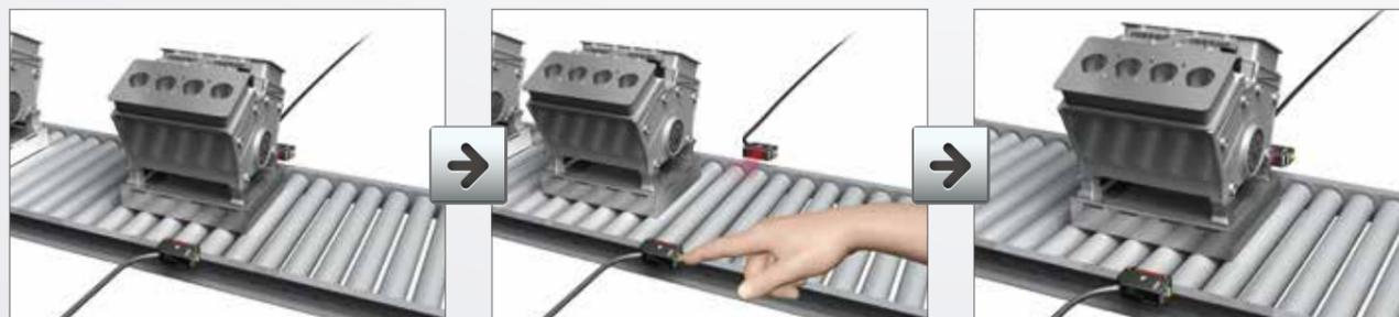
Reflected light passes through gaps in the target object, causing detection errors.
