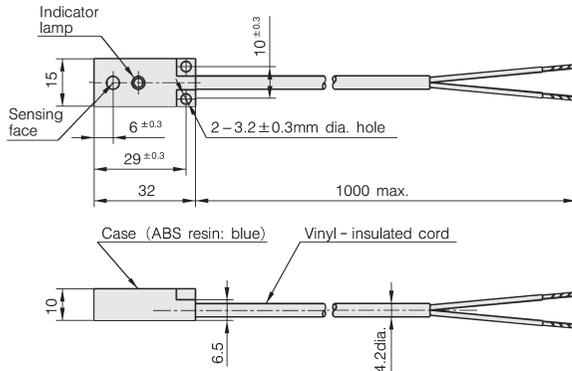
Vinyl-insulated cord (oil-resistant, bend-resistant type: 0.3mm<sup>2</sup>, 60/0.08 dia., 2-core) 4.2mm dia
