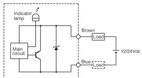
The load can be connected to either of the power supplies.
