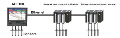
Up to 16 Network Instrumentation Modules can be registered to a single ARF100. Up to 36 recording sources can be registered, including actual analog sources (6 or 12) and communication data inputs from Network Instrumentation Modules.
